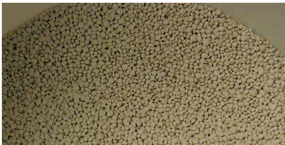
Photo 3: Ideally, the struvite will have a uniform, pellet-like shape for easy application and spreading.
