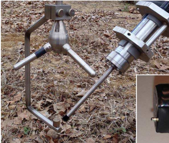
Fig. 1. Alignment of the oxygen-temperature sensor adjacent to the measuring volume of the Acoustic Doppler Velocimeter (ADV) before field deployment. The location of the measuring volume is marked by the brass cylinder on the alignment tool (at left, steel bracket) which is removed before deployment. The sensor is oriented 45° off the vertical axis of the ADV. The insert shows a close-up side view of the sensor tip with its circular oxygen-sensitive foil and thermistor. The cylindrical stem of the sensor has a diameter of 10 mm.
