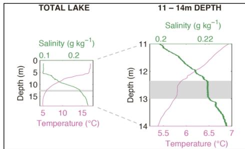
Temperature and salinity profiles at a depth of 11–14 metres in Lake Cadagno. The nearly uniform mixed layer is clearly visible at a depth of around 12.5 metres.
