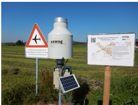
Rain measuring device at Speck airfield (Photo: Frank Blumensaat, Eawag)
