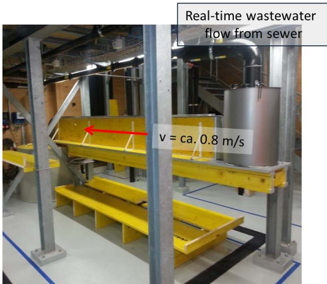
Figure SI 5. Event 3: 28.06.2017. Rain-event sampling in flow channel supplied with wastewater pumped from a main sewer.
