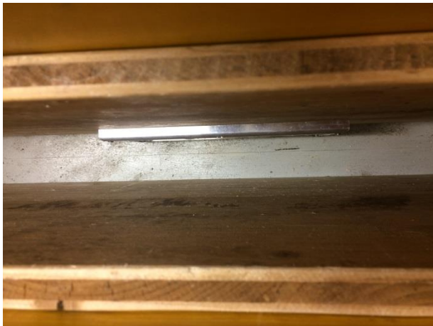
Figure SI 6. Event 3: 28.06.2017. Installation of the passive sampler setup at the flow channel wall.
