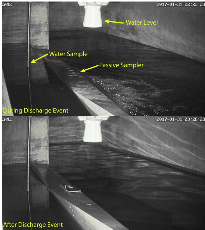
Figure SI 3. Event 2: 25.04.2017. Sampling of a sewer overflow event with sampler installed at weir crust (schematic picture from a different sampled event)
