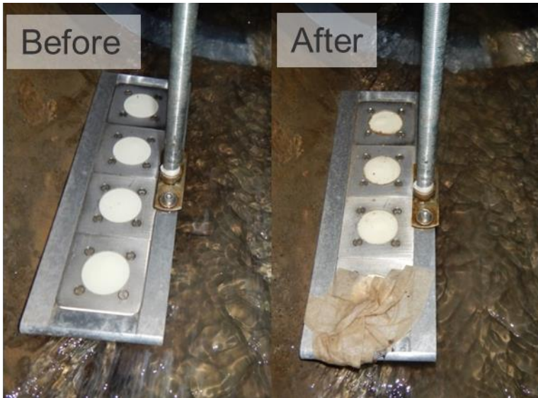
Figure SI 1. Event 1: 18.05.2016. Event-based sampling directly in the sewer. Passive sampler overflowed and auto-sampling triggered at water levels above 6cm.
