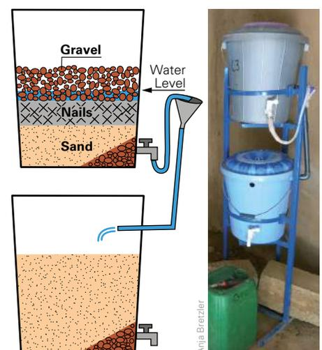
Figure 2: Cross-section of the arsenic removal filter constructed and tested in Burkina Faso.
