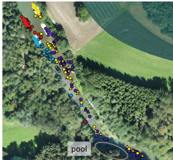
**Fig. 6.** Distribution of the RFID PIT tag equipped stones in the Sarine river. The color indicates the origin of the stones from the initial deposit. There is a pool in the bend downstream.  $D_{90}$  are indicated with a circle,  $d_m$  with a triangle.
