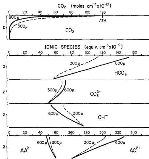
Fig. 3. Concentration profiles of different species across the stagnant boundary layer of Lake 227. The profiles represent steady state results of the model calculations for 300 and 600  $\mu$ .
