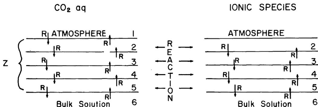
Fig. 1. A schematic representation of the multireservoir diffusion model;  $Z$  is the boundary layer thickness, and  $R$  is a transfer velocity between reservoirs.
