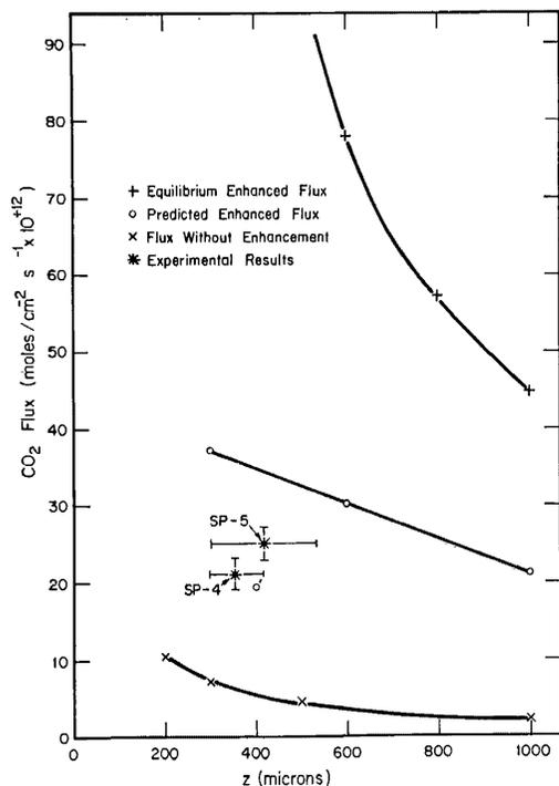
Fig. 4.  $\text{CO}_2$  flux as a function of boundary layer thickness showing calculated results for the three different cases and the experimental results.  $\circ$  is the model result solved for the chemistry of the simulation experiment.
