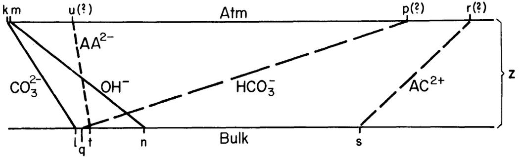
Fig. 2. Species gradients across the Lake 277 boundary layer at chemical equilibrium. Concentrations are given in Table 5 and calculation procedures in Table 7 (the lower boundary values are relative concentrations in equivalents).
