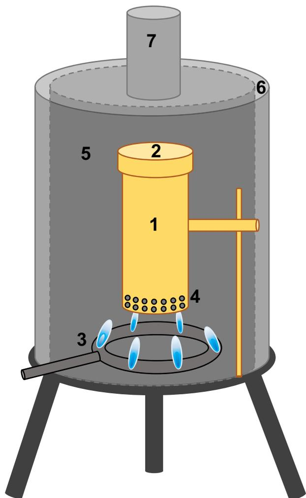
**Fig. 1** Schematic diagram of pyrolysis batch reactor. (1) Steel cylinder ( $\text{\O}$ :76.1 mm, h:300 mm) containing feedstock (2) screw cap (3) ring burner run with propane gas initiating pyrolysis process (4) perforations for the escape of pyrolysis gases (5) aluminium cover ( $\text{\O}$ :353 mm, h:500 mm) (6) insulation wool 50 mm (7) outlet for exhaust gases (8) temperature sensor
