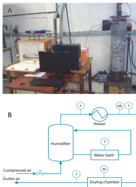
**Figure 4.19** A) the custom-designed convective drying rig (photo: UKZN PRG) and B) a schematic representation of the convective drying rig, F: air-flow measurement; T: temperature measurement; M: mass measurement; HR: relative humidity measurement.
