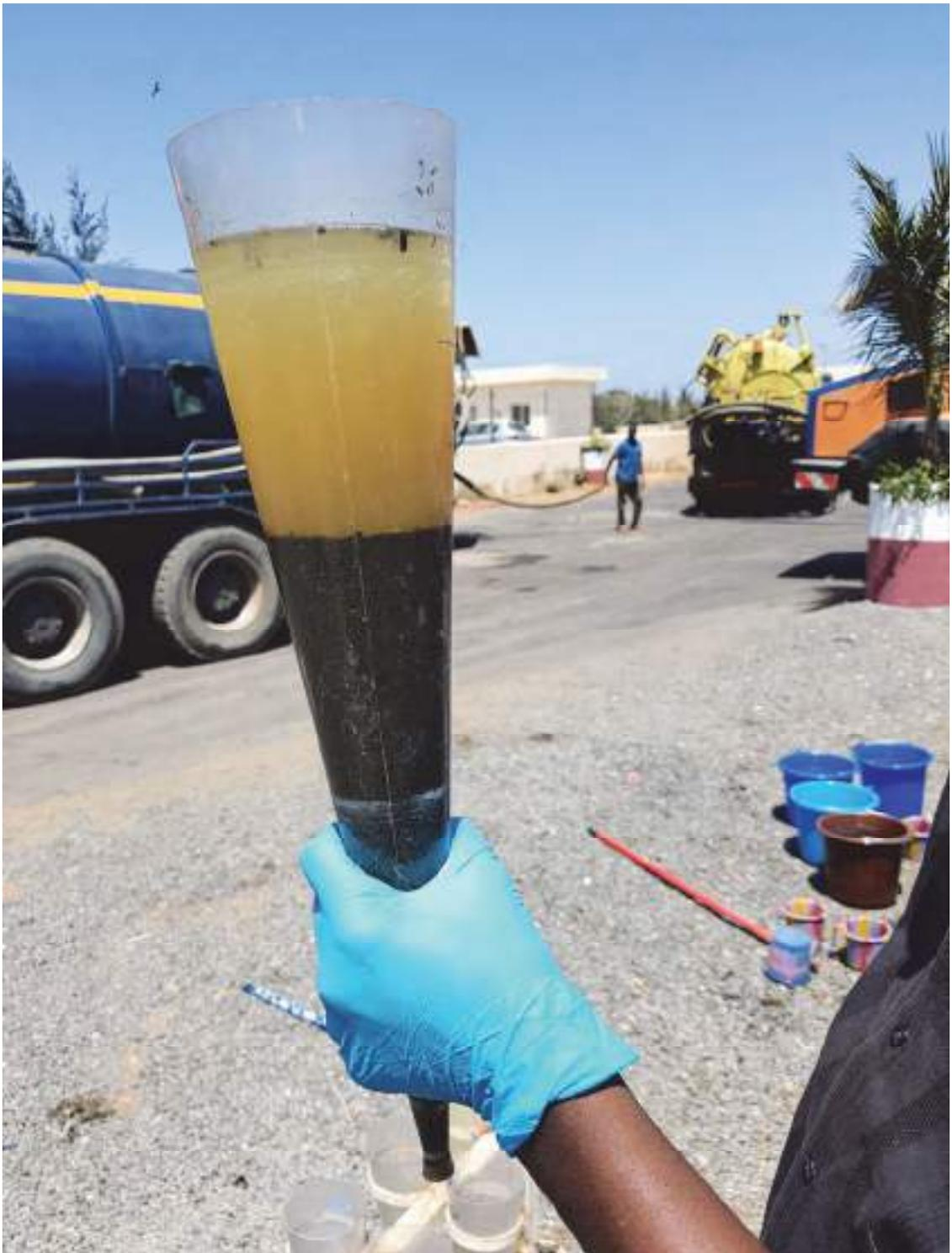
Figure 4.27 Settling tests following faecal sludge conditioning experiments at Niayes FSTP, Dakar, Senegal (photo: Eawag).
