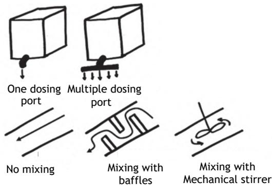
**Figure 4.11** Diagram representation of the different conditioner dosing and mixing configurations evaluated by Sanivation.
