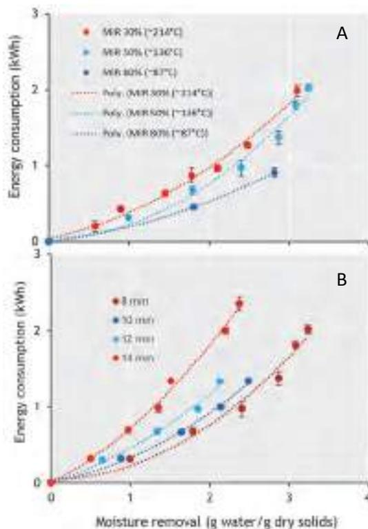
**Figure 4.22** A) Plot of moisture removal vs energy consumption at varied medium-wave infrared intensities (MIR). MIR of 30, 50 and 80% equals infrared irradiance of 6, 24, and 34 kW/m<sup>2</sup>, respectively, and B) plot of moisture removal vs energy consumption at varied pellet diameters.
