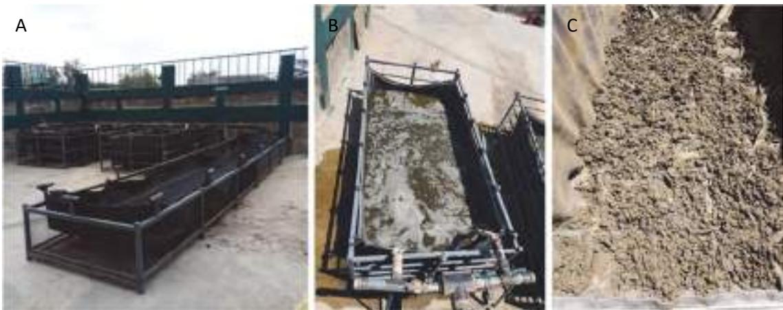
**Figure 4.10** A) a geotextile skip setup at the pilot facility; B) a geotextile skip being loaded with conditioned faecal sludge; C) dewatered sludge ready to be unloaded from a geotextile skip (photos: Sanivation).
