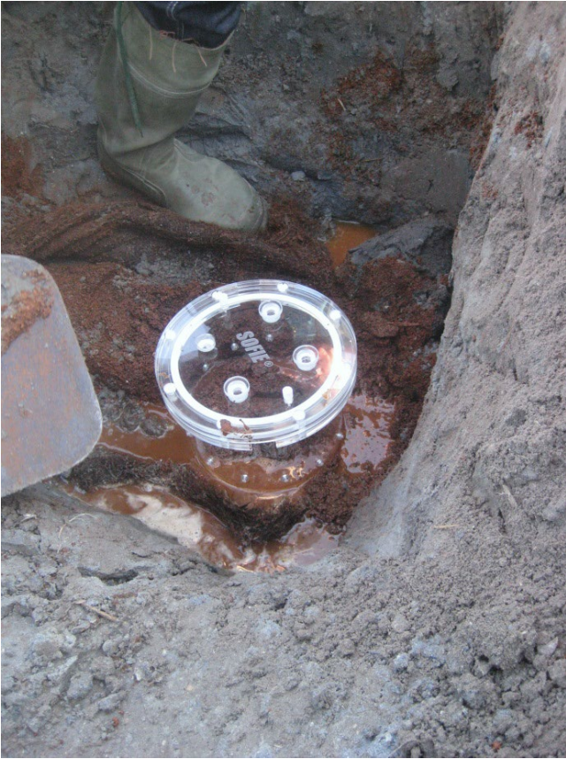
Fig. S1. In-situ field sampling of the Fe-coated sand envelope with the SOFIE® cell.
