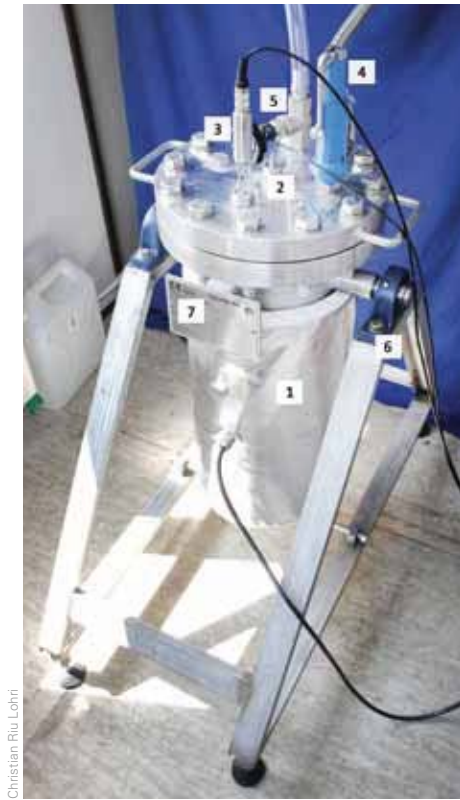
Photo 1: Prototype HTC reactor. (1: Heating mantle, 2: Temperature sensor, 3: Pressure sensor, 4: Overpressure valve, 5: Drain valve, 6: Bearing, 7: Identification plate with CE sign)
