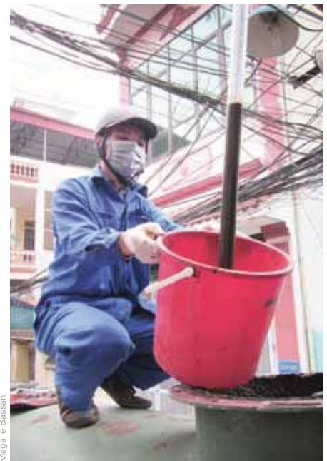
Photo 2: Sampling from the access port at the top of a truck.
