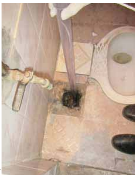
Photo 1: Core sample being taken from a septic tank.
