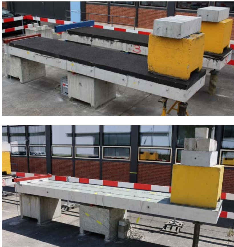
Figure 5. Test setup: (Top) Strengthened slabs with non-prestressed strips and mastic asphalt; (Bottom) Strengthened slab with prestressed strips and a protection paint layer.
