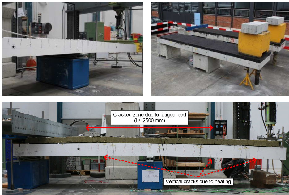
Figure 4. Cantilever static loading test to failure (upper left), cantilever test with asphalt under sustained load (upper right), cantilever fatigue test under elevated temperature (with heating mats) (bottom).
