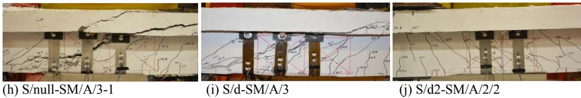
Figure 3: Crack Patterns for the tested shear-critical beams
