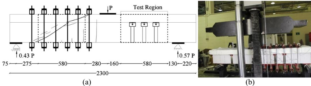
Figure 2: External Protection system and test setup; a) Schematic drawing and dimension of the external protection system and b) test setup.
