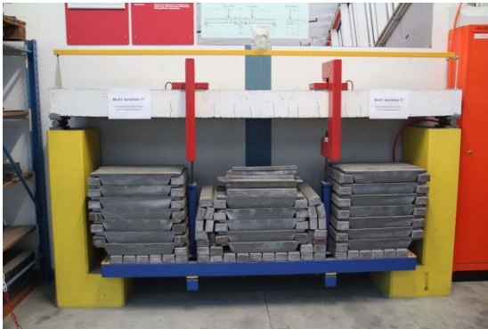
Figure 4: Long-term test at Empa: RC beam strengthened with a bonded steel plate under a sustained load.
