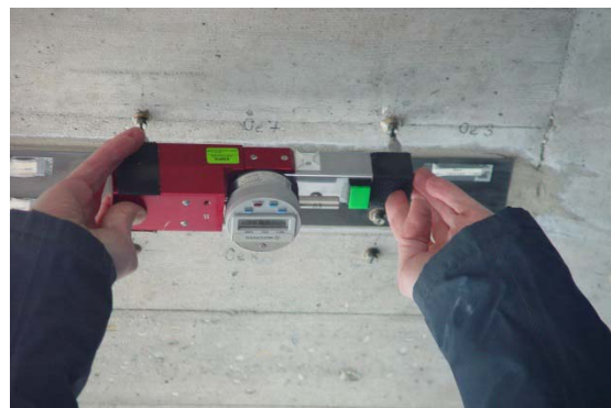
Figure 12: Mechanical strain gauge, which is used for the measurements.
