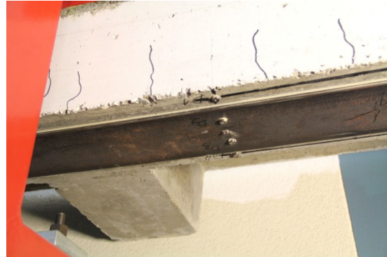
Figure 7: Bottom side of the beam in the year 2015. Surface corrosion is visible on the steel plate.
