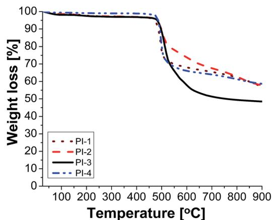
Fig. 2 TGA curves of polyimides PI1–PI4 in nitrogen.
