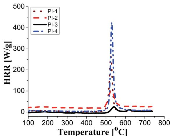
Fig. 5 HRR curves of PI1–PI4 from PCFC data.
