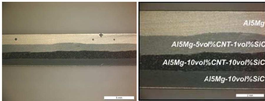
**Fig. 1.** Cross section of the multilayer plate showing the different layers and their interfaces.
