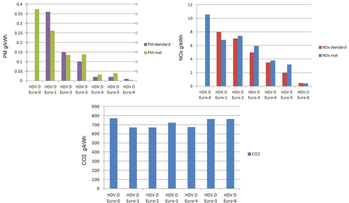
Fig. 4. PM, NO<sub>x</sub> and CO<sub>2</sub> emissions produced by typical engines for heavy duty vehicles (Harald Jenk 2015).
