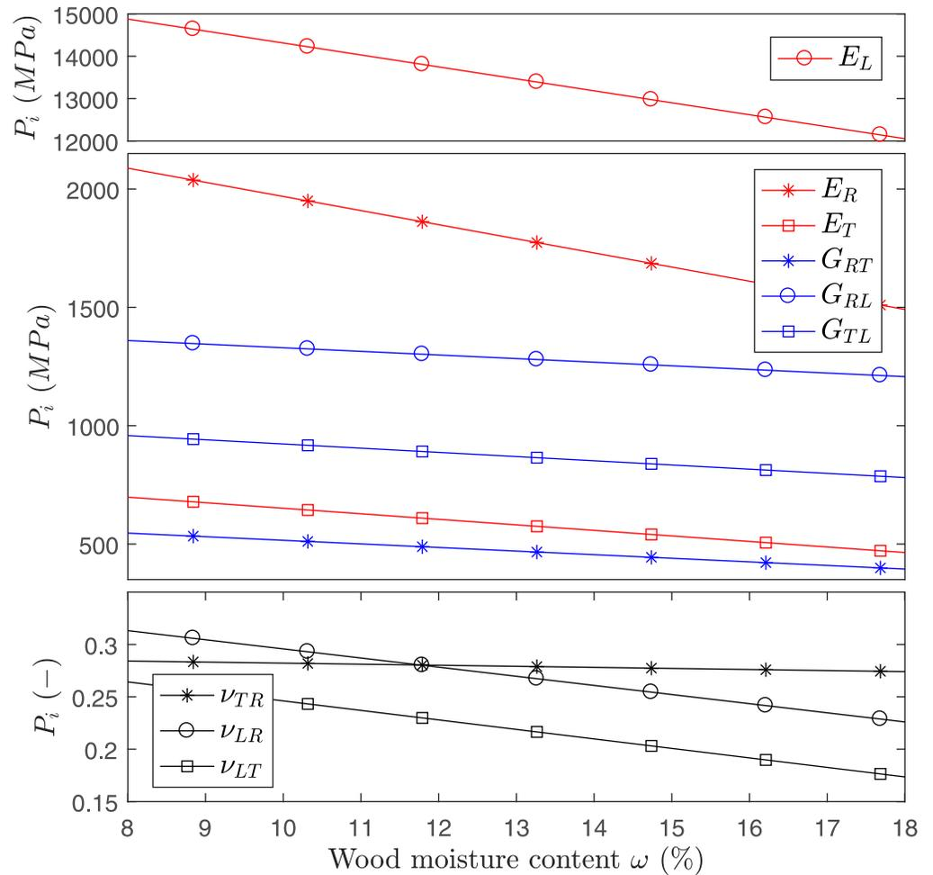
**Fig 1. Elastic properties for European beech.** Properties  $P_i$  as function of moisture  $\omega$  as found in Refs [14] and [15]. The moisture interval [8%, 18%] roughly corresponds to a relative humidity range of [35%, 85%] (adsorption at 85% and desorption at 35%).
