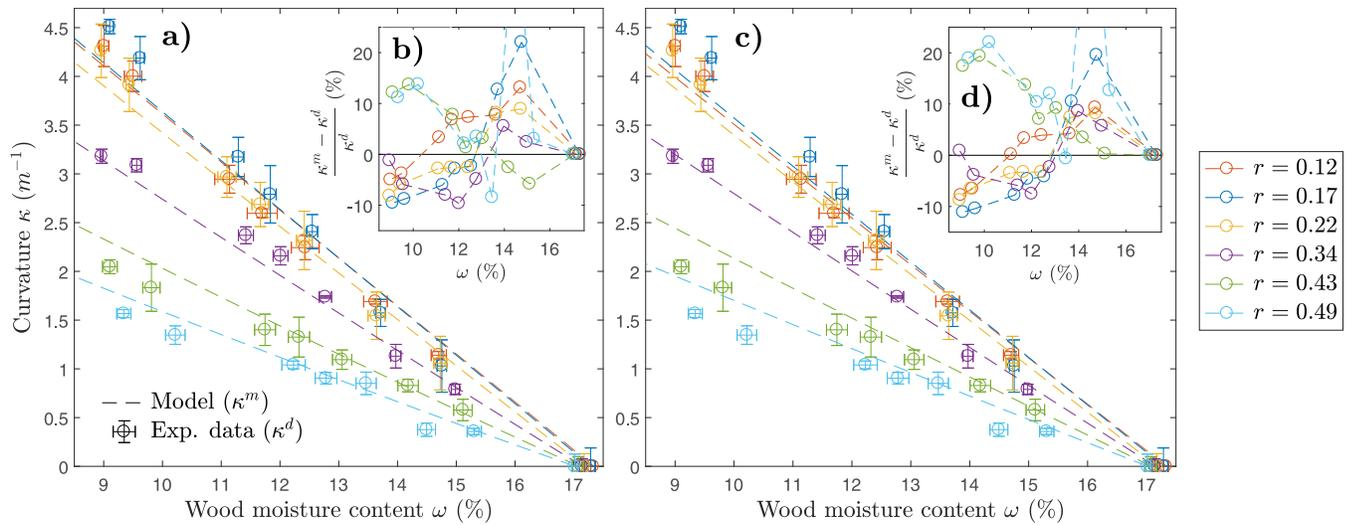
**Fig 3. Model curvature ( $\kappa^m$ ) vs. experimental validation data ( $\kappa^d$ ).** a) Plane strain model versus data (error-bars denote positive and negative standard deviations); b) Error in prediction of plane strain model with respect to experimental data ( $(\kappa^m - \kappa^d)/(\kappa^d)^{-1}$ ); c) Plane stress model versus data; d) Error in prediction of plane stress model with respect to experimental data.
