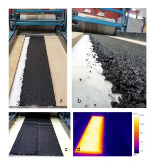
Figure 1. Detail of compaction process for design A joints. First lane after compaction without lateral confinement (a, b). Real image (c) and IR-image (d) with the temperature distribution for a hot-cold joint during the compaction of the second lane.
