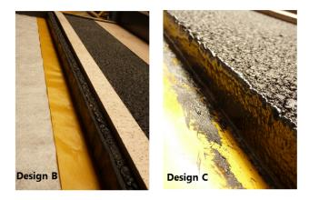
Figure 2. Self-adhesive tape applied to the interface in joints design B (left) and bituminous sealing applied to the interface for joints design C (right).
