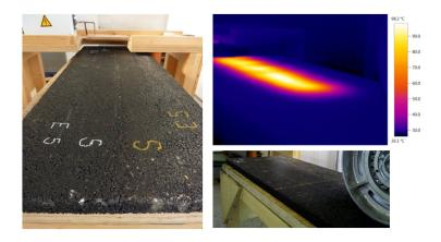
Figure 4. Details of the induction heating treatment and extra-compaction of the joint design E. 254x190mm (96 x 96 DPI)
