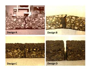
Figure 6. Details of fractures for different joint designs. 254x190mm (96 x 96 DPI)
