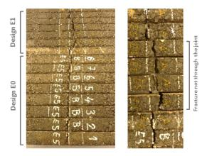
Figure 7. Details of fracture path in specimens with joint designs E0 and E1.  $254 \times 190 \text{mm} \; (96 \times 96 \; \text{DPI})$
