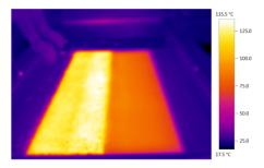
Figure 3. IR-image at the beginning of the compaction of a slab with joint design D.  $254 \times 190 mm \; (96 \times 96 \; DPI)$
