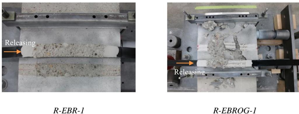
Figure 4. Failure mode of EBR and EBROG.
