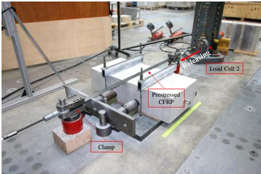
Figure 1. Test setup for the prestress force-release tests.
