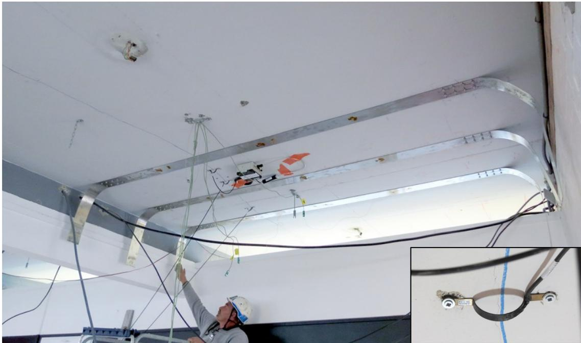
Figure 3. Strengthened RC slab to reduce crack width and measurement with Omega-deformation gauges
