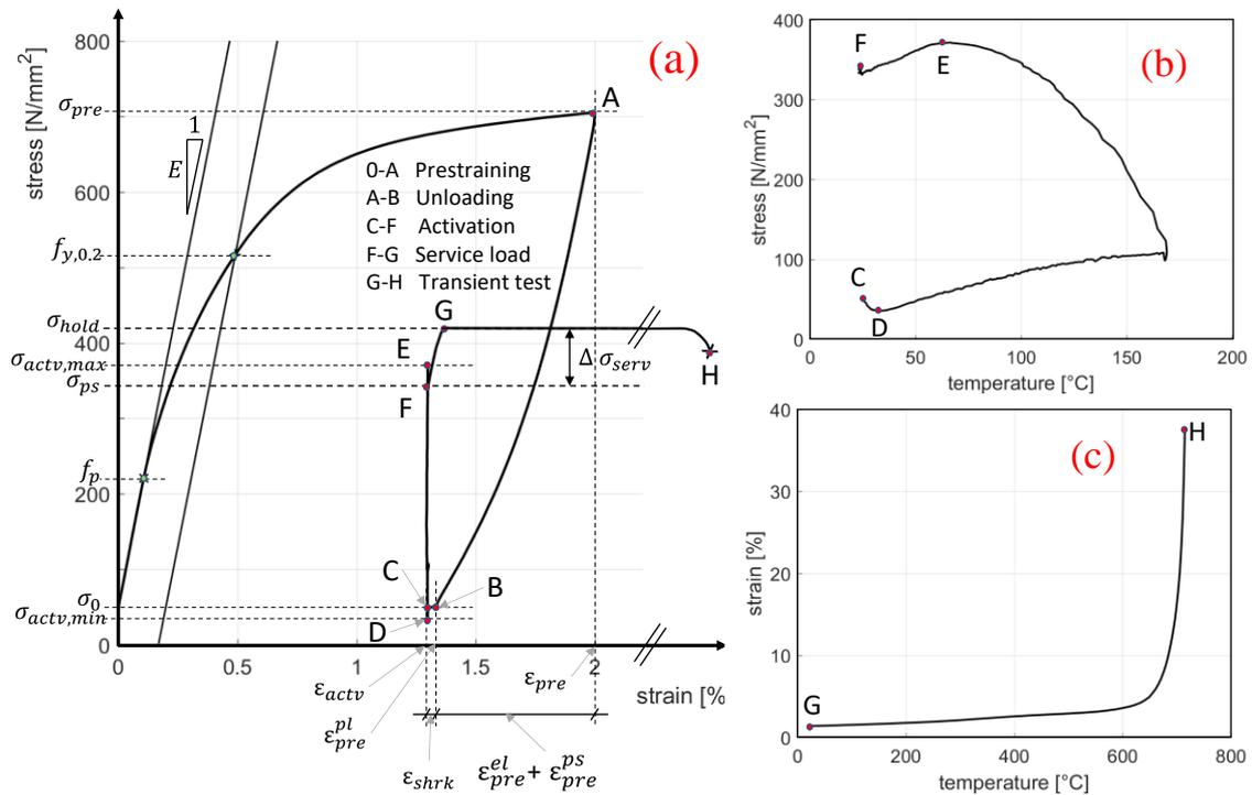
Figure 2. Test procedure of the transient tests on the activated Fe-SMA strips: a) the stress-strain behavior (during pretraining, unloading, activation process, application of the service load and the transient test) with the indication of the mechanical properties, b) the stress-temperature behavior during the activation process, and c) the strain-temperature behavior during the total transient deformation test (Ghafoori et al., 2019)
