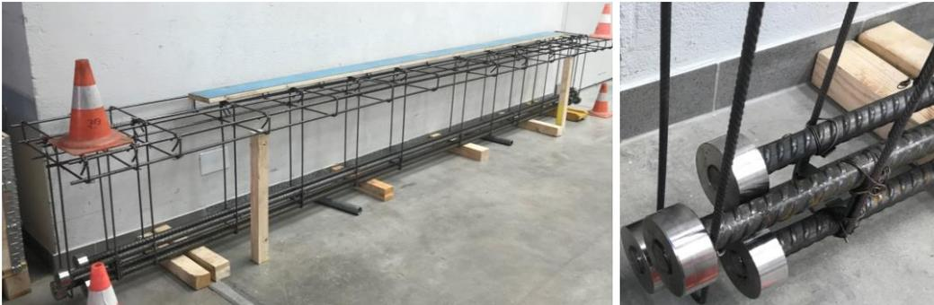
Figure 6: Left: A photo of the internal reinforcement for Beam No. 1, Right: A photo of the end anchorage system for the longitudinal bars of diameter 30 mm.
