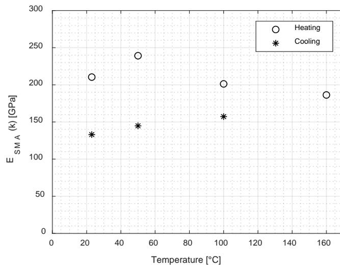
Figure 8 The evolution of  $E_{SMA}(k)$  during activation.
