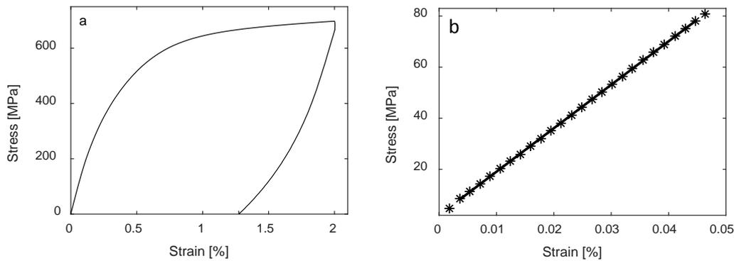
Figure 5(a) Stress as a function of strain during pre-straining to 2%; (b) The black line is linear fitting (regression line) in the stress range from 5 to 80 MPa.
