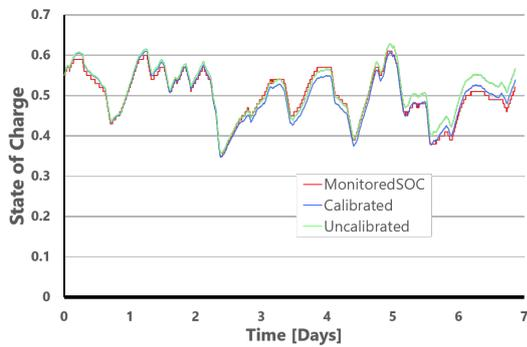
**Figure 1.** Comparison of SOC for the lithium ion battery.
