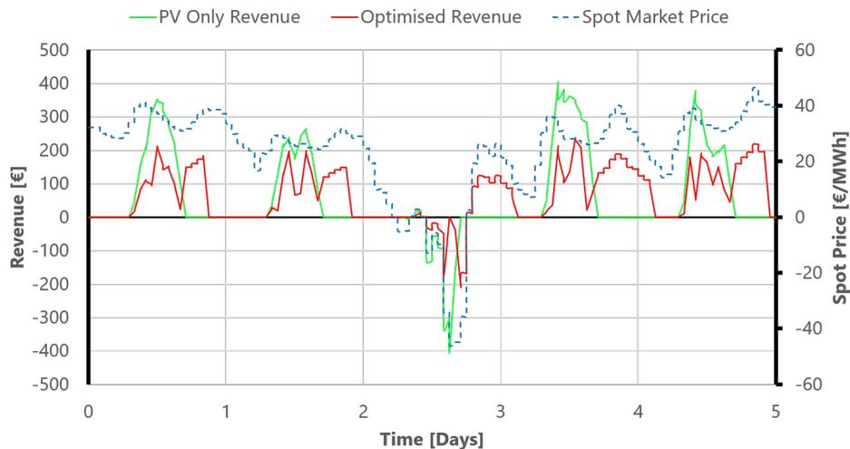
**Figure 5.** Optimized solution to shift the export of electricity using battery storage
