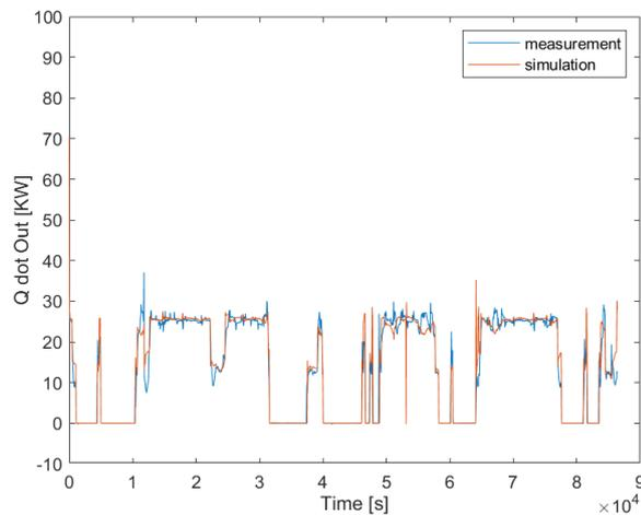
**Figure 4.** Simulating the output of a heat pump
