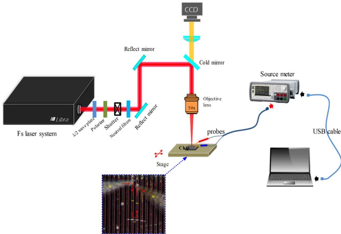
**Figure S1.** Schematic of the experimental set up. The fs laser beam is attenuated before entering the optical system. Using optical microscopy, the laser beam is further focused and directed to the selected points in the SiC-Au circuit. After laser irradiation, the Au electrodes were connected with two (W) probes, which are implemented in a computer controlled electrical measurement platform.
