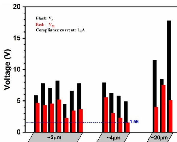
**Figure S2.** Statistical results of 'write' ( $V_S$ ) and 'maintain' ( $V_M$ ) voltages in SiC-Au circuits (before laser processing) having different bridge lengths. The difference between 'write' and 'maintain' voltages is more stable when the nanowire bridge is shorter. A low 'maintain' voltage is possible for a SiC-Au circuit when the bridging length is  $< 4 \mu\text{m}$ .
