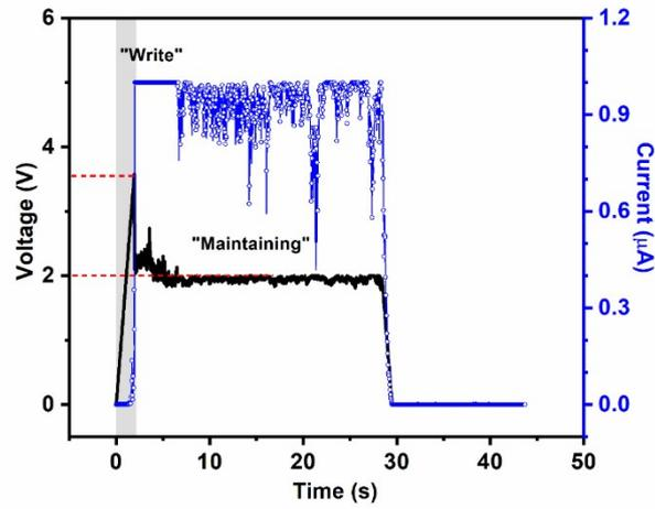
**Figure S4.** Current response of the 2  $\mu\text{m}$  SiC-Au circuit (before laser processing) under a programmed voltage bias. The 'write' process is completed rapidly in this short-bridged structure.
