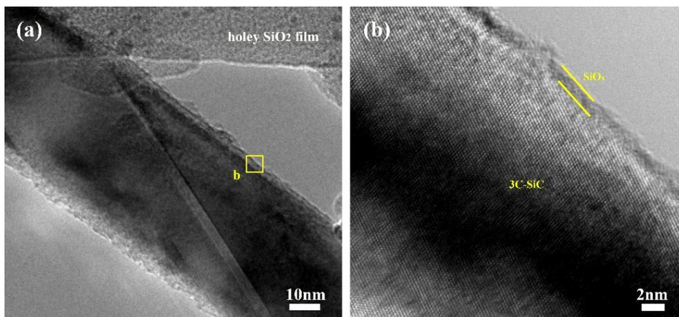
**Figure S5.** (a) TEM image of a core/shell SiC/SiO<sub>2</sub> nanowire after fs laser irradiation. (b) Magnified TEM image at the edge of nanowire. The oxide thickness is reduced to ~ 1.1 nm after irradiation. Laser fluence: 20 mJ/cm<sup>2</sup>. Duration: 5 s.
