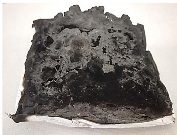
**Fig. S7.** Intumescence char residue after cone calorimetry test for **EPO2Si\_DP2P\_Mel** [5, 6].
