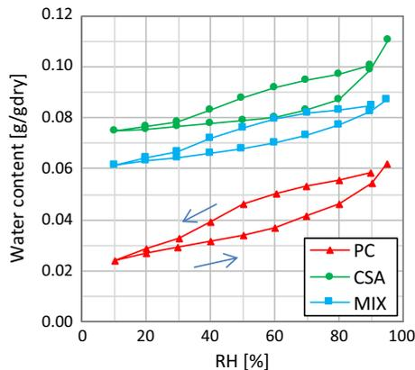
**Fig. 2** Sorption isotherms at 20 °C at 182 days for the three investigated mixtures in the range 10–95% RH. The water content was calculated with reference to the dry specimen mass at 0% RH and 40 °C
