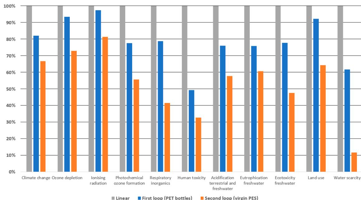
**Figure 3.** Environmental impact comparison between the linear product system (grey) and the first (blue) and second loop (orange) product systems.
