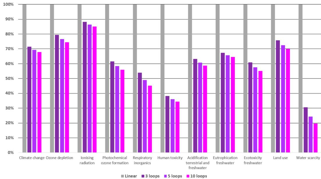
**Figure 4.** Environmental impact comparison between one linear product system and the average impacts of three, five and ten wear2wear™ product systems. Each of the product systems contain one first (blue) loop. The remaining product systems are second (orange) loops.
