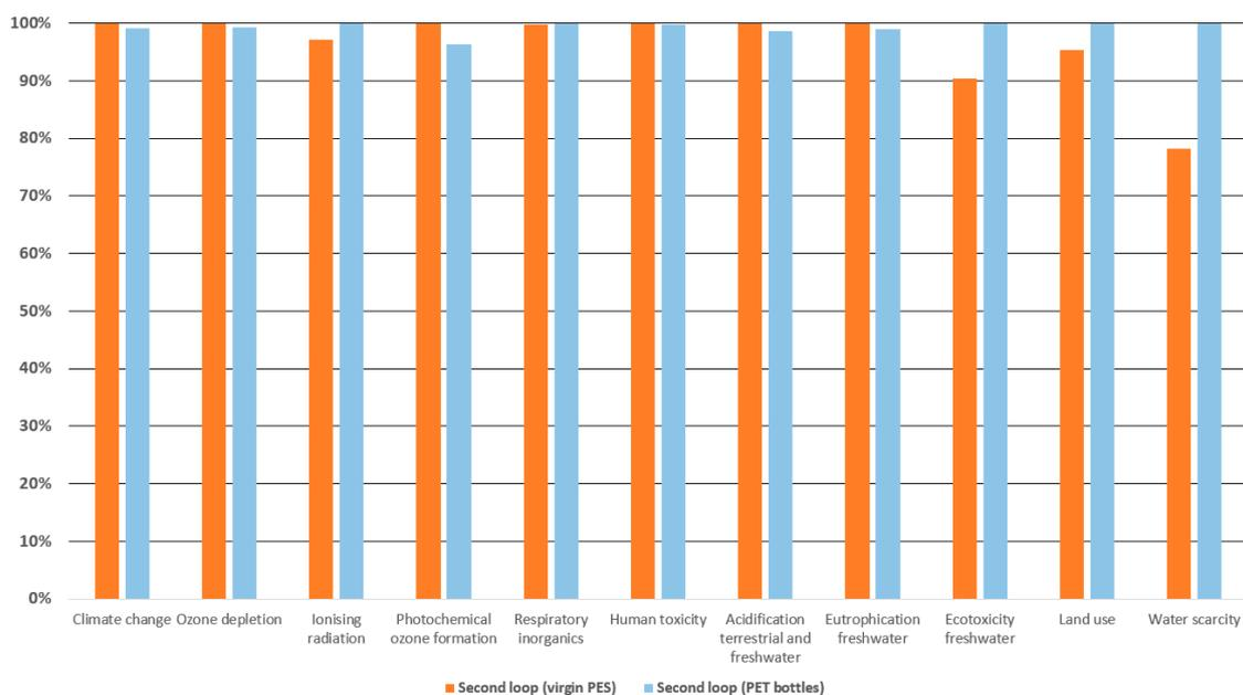
**Figure 5.** Impact comparison between the second loop product systems once with virgin PES and once with PET bottles as the main input for fiber production.
