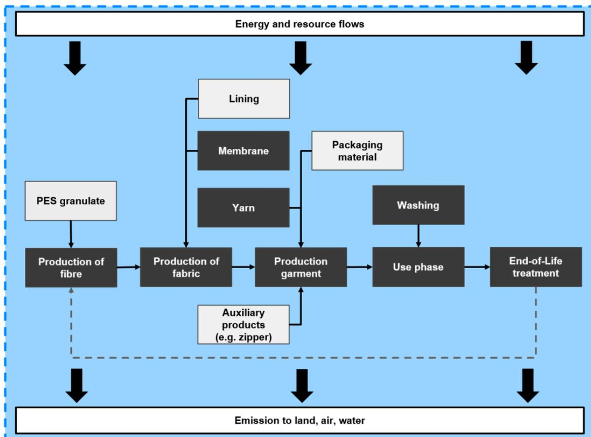
**Figure 1.** The system boundaries as set for this study. All the life cycle stages are included for the production of a three-layer laminate jacket. For the black boxes, primary data is collected directly from the partner companies. For the four grey boxes, secondary data from the ecoinvent database is utilized together with assumptions made by the partner companies (e.g., how much packaging is required) because primary data from the corresponding subcompanies are not (entirely) available.
