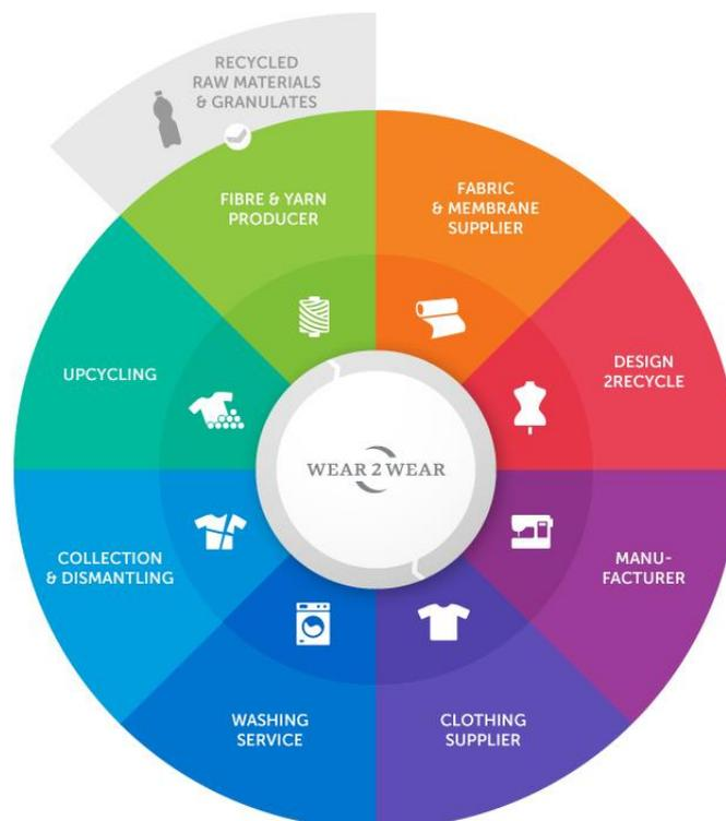
**Figure 2. The wear2wear production loop. Starting from the light green field, the fibres are spun either from virgin PES or recycled granulate. The fabric is a three layered laminate just made of PES to guarantee optimal recycling at the EoL, where new fibres are made again from remolten granulate (wear2wear™, 2020).**
