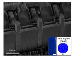
Tensile bar extensions and pillar compressions under HSR conditions
