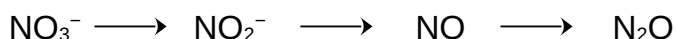
Fig. 2. Reaction sequence occurring during denitrification by Pseudomonas aureofaciens : nitrate ( NO_3^- ) is reduced through nitrite ( NO_2^- ) and nitric oxide (NO) to N_2O .
