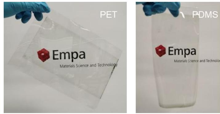
Figure S1. Digital photographs of  $\text{Ti}_3\text{C}_2\text{T}_x$  TCEs on PET and PDMS substrates.
