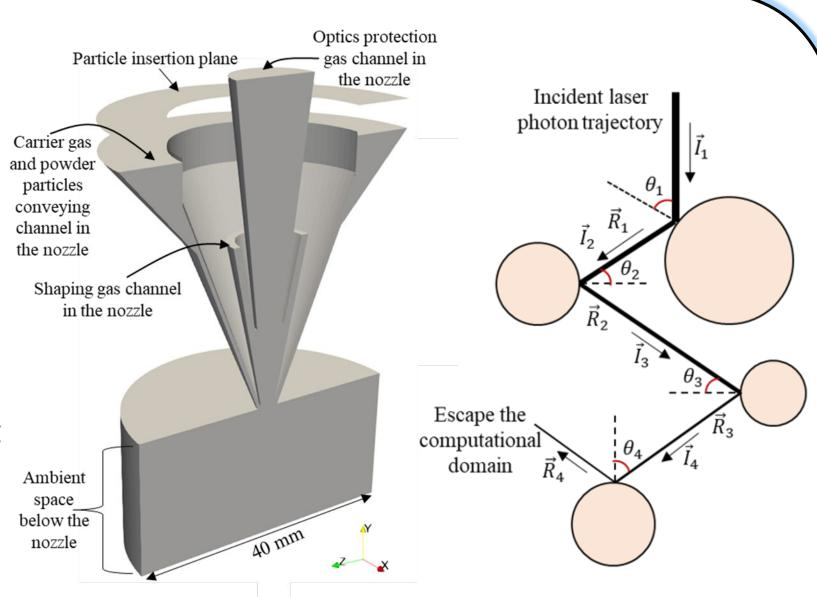
Computational domain for Schematic showing the multiple reflection of laser photon CFD-DEM
