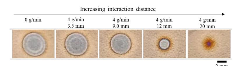
Influence of laser beam shadowing on the melt pool morphology (Titanium substrate) for different laser-particle interaction length
