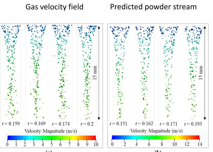
Temporal evolution of the powder stream as it emerges from the nozzle outlet predicted by four-way coupled CFD-DEM modeling (a) case P2, and (b) case P3
