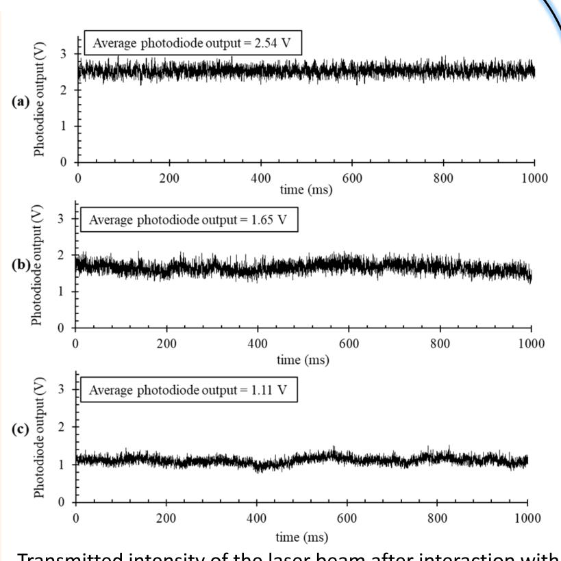
Transmitted intensity of the laser beam after interaction with the powder stream (a) Only laser (no powder stream), (b) 8 mm interaction length, and (c) 16 mm interaction length
