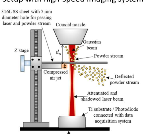
Optical breadboard mounted on DED Z-stage system for measuring laser beam attenuation
