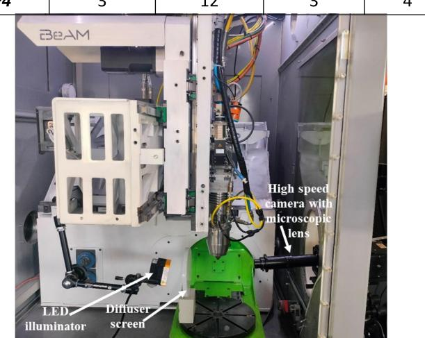
DED setup with high-speed imaging system
