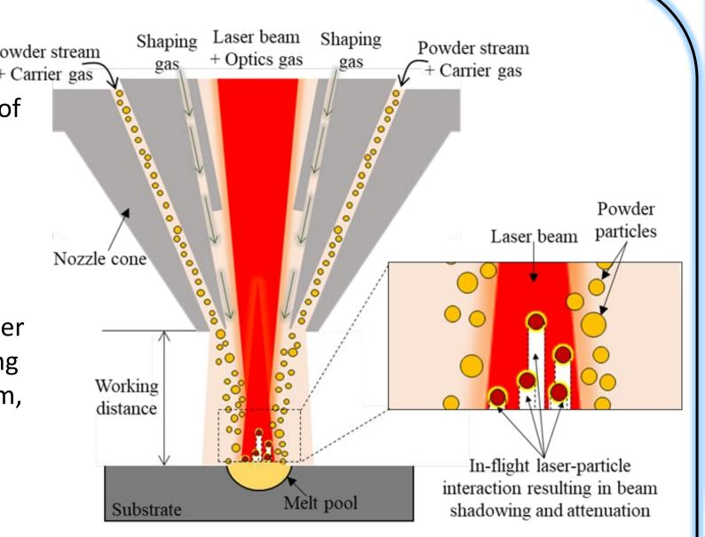
Schematic of the coaxial laser-based DED process
