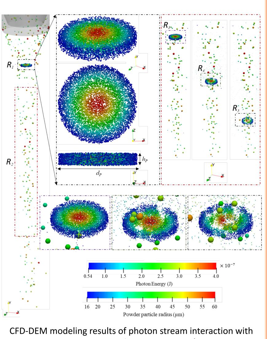
powder particles for case P2 (shaping gas = 3 l/min, optics gas = 3 l/min, carrier gas = 3 l/min, and powder feed rate = 4 g/min).
