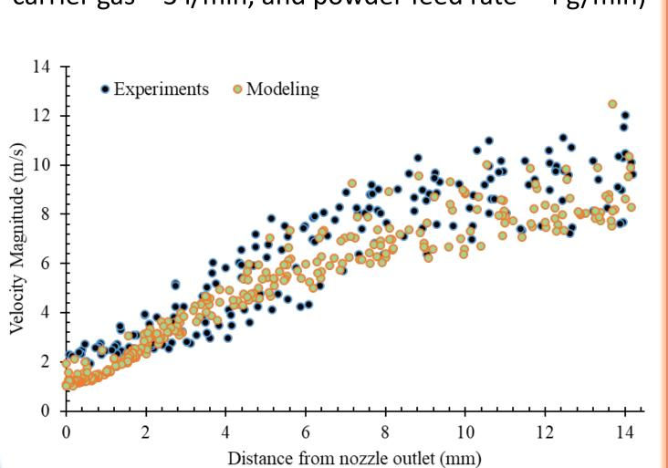
High-speed imaging and modeling results (shaping gas = 3 l/min, optics gas = 3 l/min, carrier gas = 3 I/min, and powder feed rate = 4 g/min)
