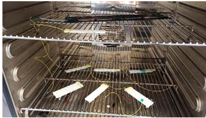
Figure 2. Setup for resin CTE measurement via DFOS.
