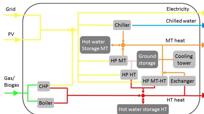
Figure 1: Energy hub of the Empa research facility
