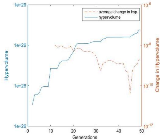
Figure 3: Hypervolume of the Pareto front and the change in hypervolume for the bi-level optimisation
