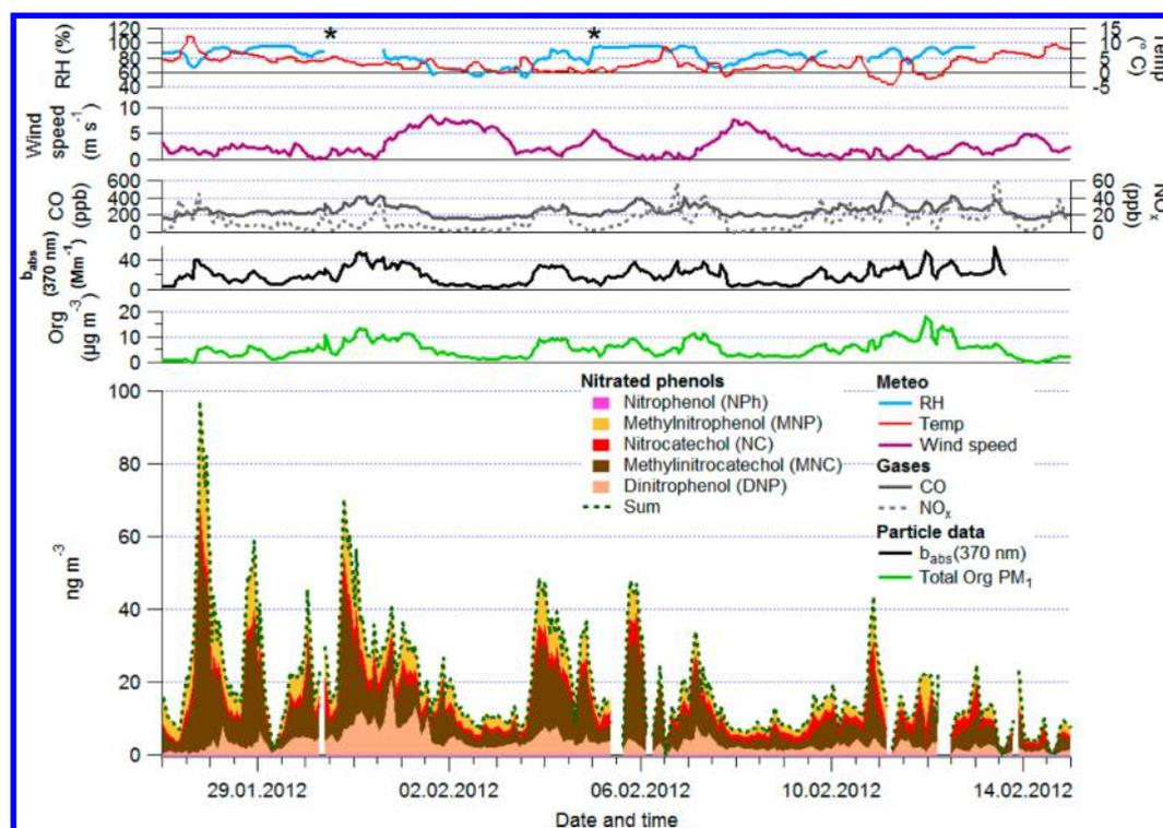
**Figure 1.** Time series of ambient temperature (Temp) and relative humidity (RH), NO<sub>x</sub>, CO, the fraction of *b*<sub>abs</sub> measured with an aethalometer at 370 nm (*b*<sub>abs</sub>(370 nm)), total organic PM<sub>1</sub>, and particulate nitrated phenols (stacked) as identified by the CIMS during the ClearLo campaign in Detling. The asterisks denote snow fall incidents.
