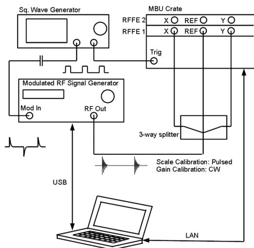
Figure 11: Calibration Set-Up.
