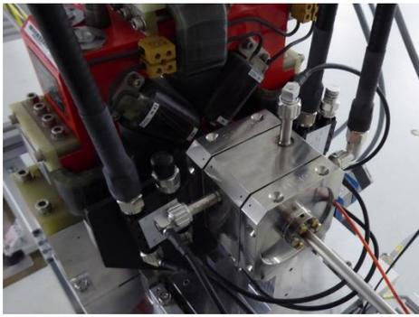
Figure 7: 8mm Undulator BPM Pickup at SwissFEL.
