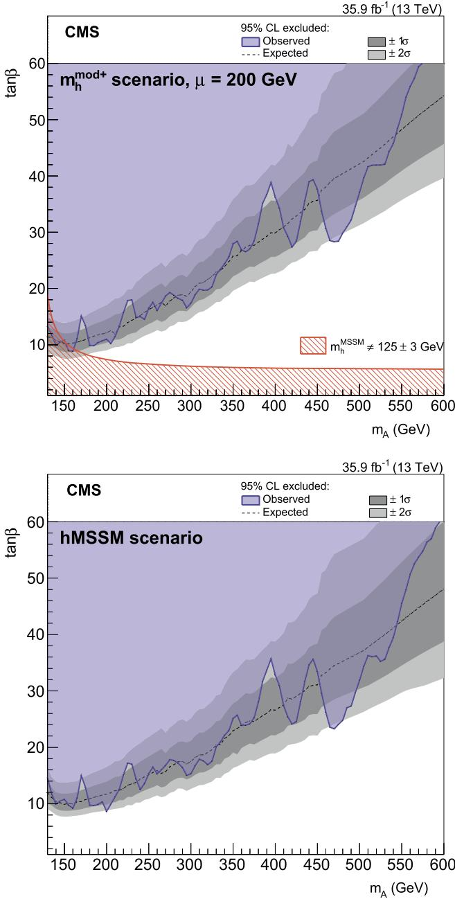
**Fig. 5.** The 95% CL expected, including the 68 and 95% CL bands, and observed upper limits, on  $\tan\beta$  as a function of  $m_A$  for the  $m_h^{\text{mod}+}$  (upper) and the hMSSM (lower) scenarios of the MSSM. The observed exclusion contour is indicated by the purple region, while the area under the red curve is excluded by requiring the neutral h boson mass consistent with  $125 \pm 3$  GeV.
