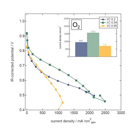
Flow: 0.2 L/min H<sub>2</sub> and O<sub>2</sub>; 100%RH; OCV vs 0.3V; 80°C 5cm<sup>2</sup> cell
