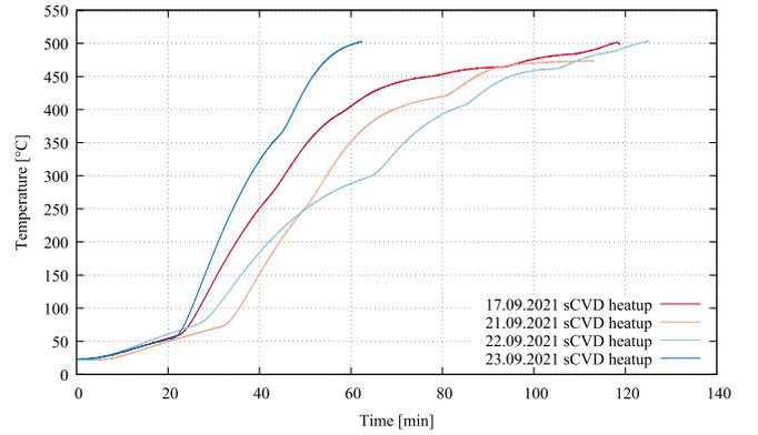
Fig. 4. Temperature as function of time for the 4 independent TCT measurement campaigns with the sCVD diamond sensor.
