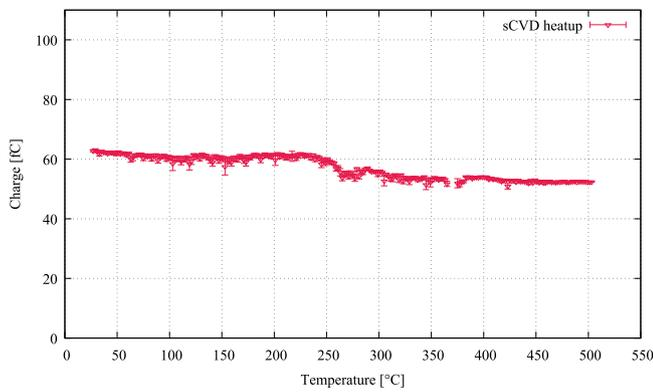
Fig. 9. Charge yield as function of  $T$  from the spectroscopic measurement of the 140  $\mu\text{m}$  thick sCVD diamond sensor. A drop is observed around  $T = 260$   $^{\circ}\text{C}$ . The charge yield at 500  $^{\circ}\text{C}$  is about 83%.
