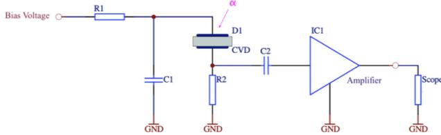
Fig. 2. Circuit diagram for the measurement setup. The  $\alpha$ -particles entered the sensors through the bias electrode and the signals were read out via the ground electrode of the sensors.
