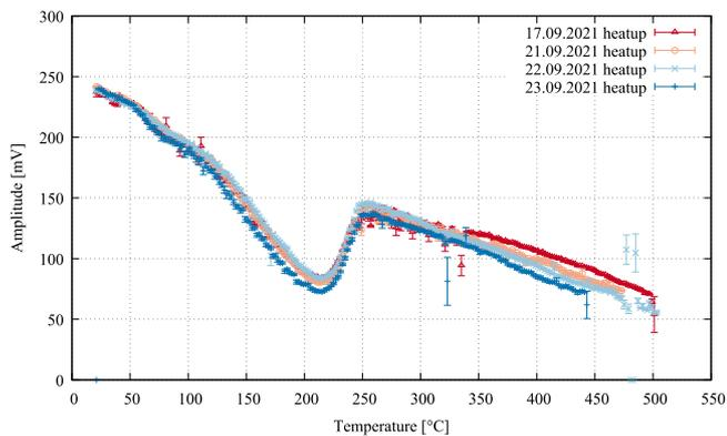
Fig. 6. Amplitudes of  $\alpha$ -particle-induced TCT-signals as function of  $T$  for the sCVD diamond sensor. The overall decrease of amplitude and the non-linearity for  $T < 260$   $^{\circ}\text{C}$  matches the characteristic of the signal FWHM.
