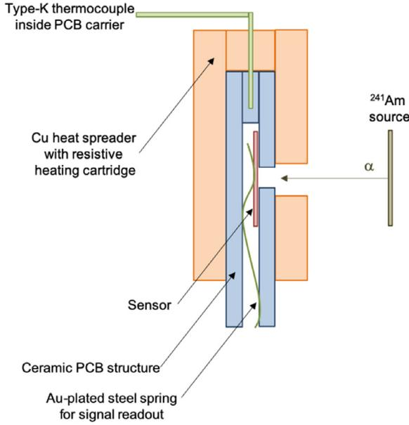
Fig. 1. Schematic of the experimental setup as installed inside the vacuum chamber.
