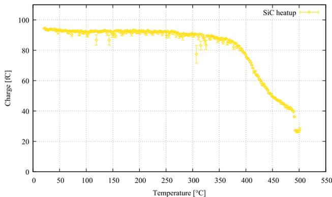
Fig. 10. Charge yield as function of  $T$  from the spectroscopic measurement of the 4H-SiC sensor. From 370  $^{\circ}\text{C}$  onwards, the charge yield drops by approximately 70% up to 500  $^{\circ}\text{C}$ .
