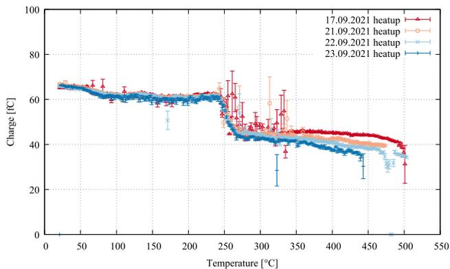
Fig. 7. Measured charge  $Q$  as function of  $T$  for the TCT-measurement campaigns with the sCVD diamond sensor. The areas of the TCT-signals were converted to  $Q$  using Eq. (1).
