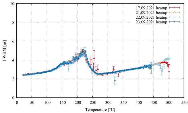
Fig. 5. FWHM of TCT-signals as function of  $T$  for the 140  $\mu\text{m}$  thick sCVD diamond sensor measuring 5.5 MeV  $\alpha$ -particles. An overall increase in  $e^-$ -drift time with a systematic non-linearity for  $T < 260$   $^{\circ}\text{C}$  is observed.
