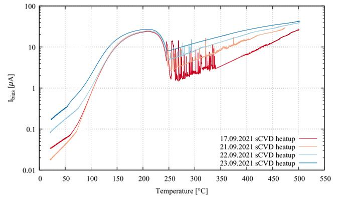
Fig. 8. Measured bias current as function of  $T$  for the sCVD diamond sensor. An overall exponential increase with a characteristic shoulder for  $T < 250$   $^{\circ}\text{C}$  is observed. The peak structures are likely measurement artefacts caused by the autoscale function of the electrometer.
