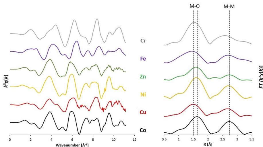
Fig. 5 (Left) EXAFS spectra of Cr, Fe, Zn, Ni, Cu, and Co for 8-cation LDH. (Right) The Fourier transform of the  $k^3\chi(k)$  taken using the range of  $k = 2.5\text{--}10 \text{ \AA}^{-1}$ . Scattering distances are uncorrected for phase-shift.
