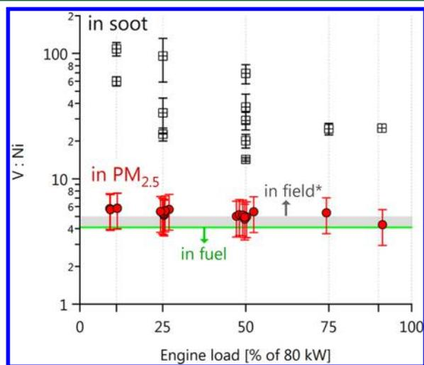
**Figure 3.** Mass ratio V:Ni in soot particles and in the  $\text{PM}_{2.5}$  of HFO exhaust. Also shown are the ranges of values measured in the fuel itself (green thin line) and in field measurements of atmospheric particles (gray shading, measured by Viana et al.<sup>78</sup>). The horizontal scatter of the  $\text{PM}_{2.5}$  data is added for clarity only. Error bars are s.e.m.
