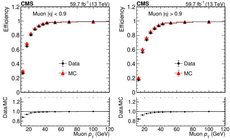
**Figure 9.** Efficiency of the prompt-muon MVA selection as a function of the muon  $p_T$  for muons with  $|\eta| < 0.9$  (left) and  $|\eta| > 0.9$  (right), for the 2018 data set with black dots and simulated DY events with red triangles. The vertical bars on the plots represent the statistical uncertainty of each measurement.
