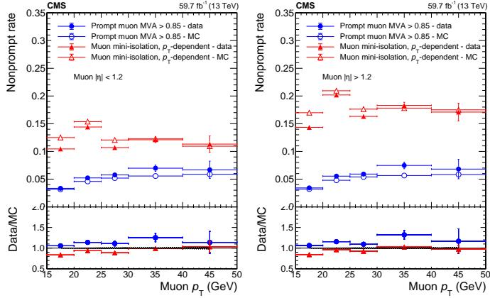
**Figure 11.** Measurement of the nonprompt-muon rate of a prompt-muon MVA (blue dots) and mini-isolation (red triangles) selection as a function of  $p_T$  for muons with  $|\eta| < 1.2$  (left) and  $|\eta| > 1.2$  (right) for the 2018 data set and simulated DY events.
