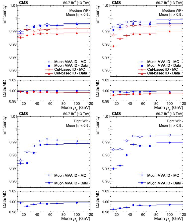
**Figure 7.** Muon identification efficiency for the medium (upper) and tight (lower) WPs as a function of  $p_T$  for muons with  $|\eta| < 0.9$  (left) and  $|\eta| > 0.9$  (right). Blue dots show the muon MVA ID performance both for the 2018 data set and DY simulation, whereas red triangles show the efficiency of the medium cut-based ID used during Run 2. The data to MC ratio is also shown. The efficiencies of the muon MVA ID are similar in both  $\eta$  regions.
