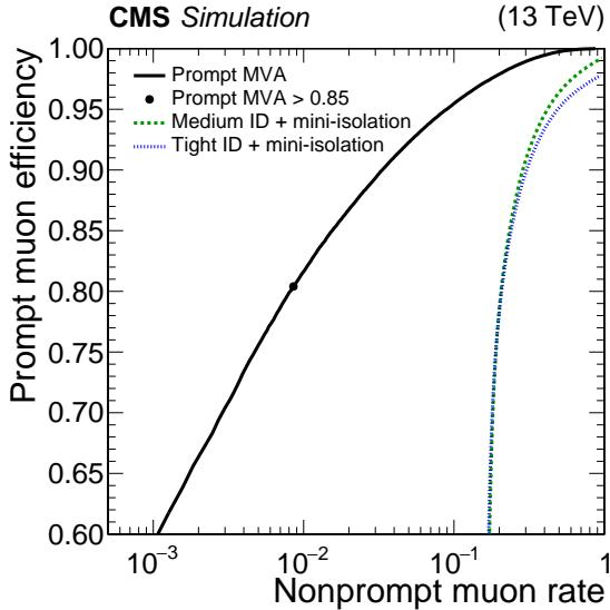
**Figure 6.** ROC curve for the prompt-muon MVA, and for the tight and medium cut-based criteria together with requirements on mini-isolation. For a set of cuts on the different discriminators, the efficiency is shown as a function of proportion of nonprompt muons passing the WP selection.
