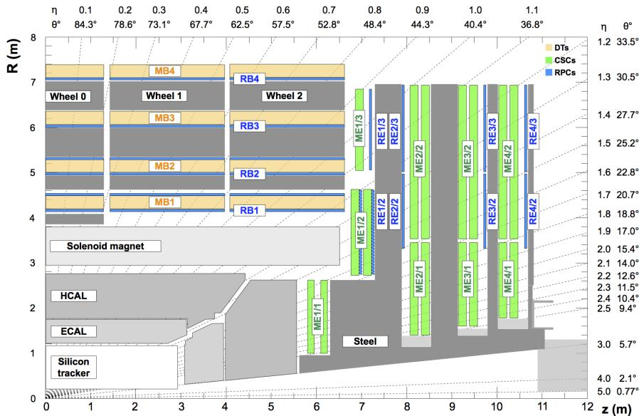
**Figure 1.** Layout of a quadrant of the CMS detector with the muon system highlighted. The chambers are named MB for muon barrel, corresponding to DT chambers, and ME for muon endcap, corresponding to CSC chambers. The RPC chambers are named RB and RE for barrel and endcaps, respectively. Reproduced from [2]. © 2018 CERN for the benefit of the CMS collaboration. CC BY 3.0.
