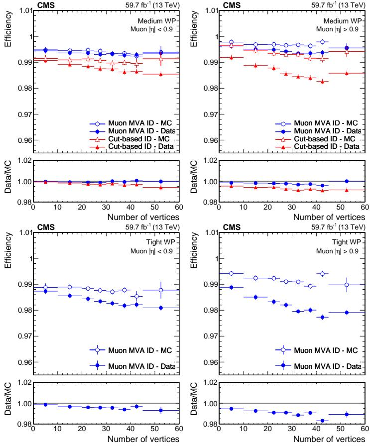
**Figure 8.** Muon identification efficiency for the medium (upper) and tight (lower) WPs as a function of PU for muons with  $|\eta| < 0.9$  (left) and  $|\eta| > 0.9$  (right). Blue dots show the muon MVA ID performance both for the 2018 data set and DY simulation, whereas red triangles show the efficiency of the medium cut-based ID used during Run 2. The data to MC ratio is also shown.
