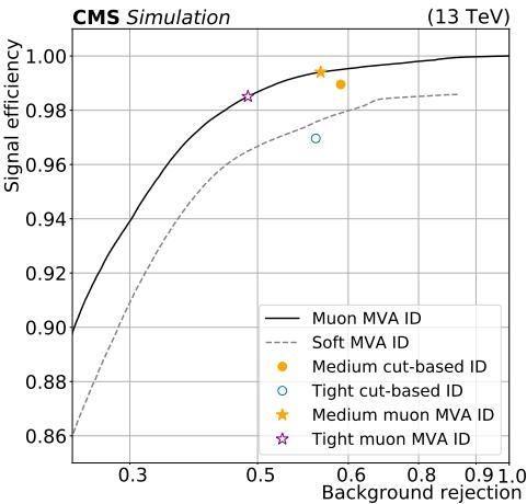
**Figure 4.** The ROC curve for muons with  $p_T > 10$  GeV for the developed general muon MVA ID discriminator (black solid line) with the selected medium and tight WPs shown as orange solid and purple open stars, respectively. Orange solid and blue open points show the medium and tight WPs of the cut-based ID. The ROC curve of the soft MVA ID [11] is also shown (grey dashed line).
