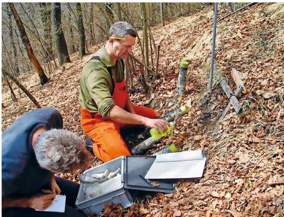
As part of the monitoring programme, LWF researchers at WSL use a tensiometer to measure the forces that a plant must overcome to be able to take up water from the soil.
