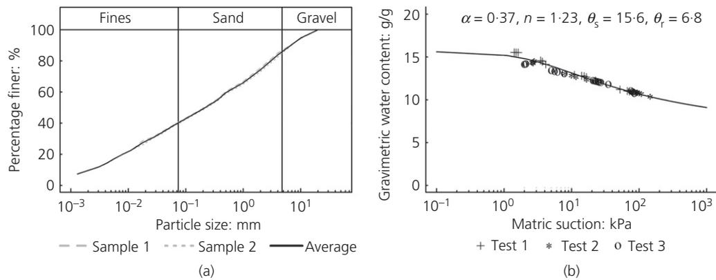
Figure 1. (a) Grain size distribution of Praettigau soil, classified as clayey sand based on USCS, obtained by a combination of wet sieving and hydrometer methods, performed on two samples from a main batch; (b) SWRC of the Praettigau soil and the fitting parameters for the equation of Van Genuchten (1980)
