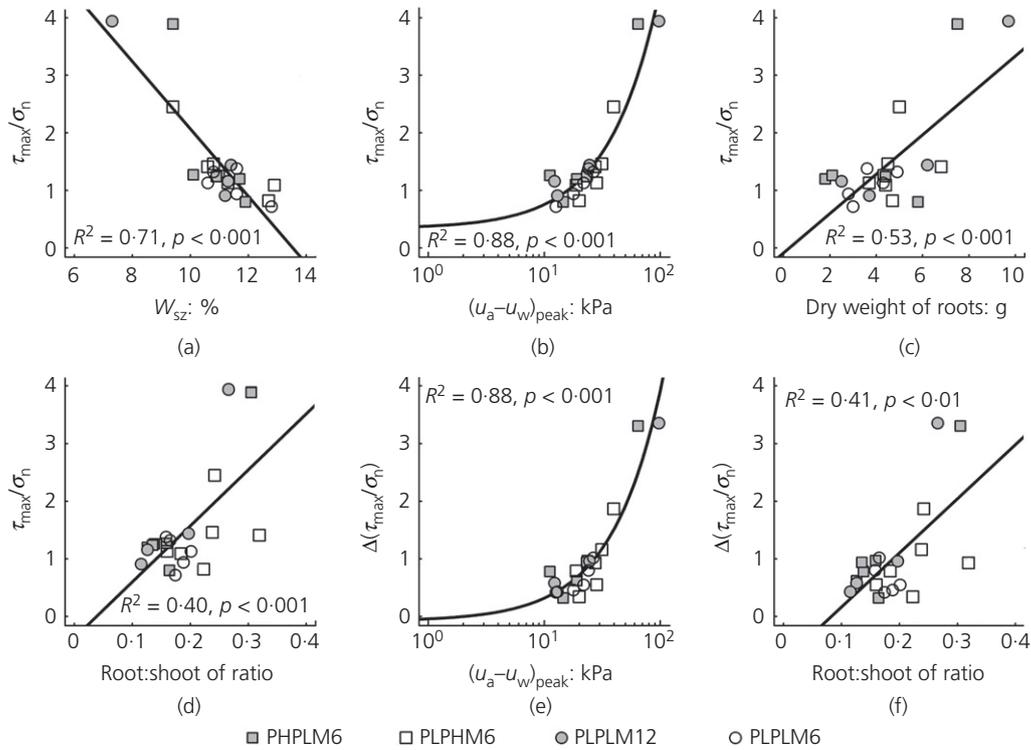
Figure 5. Relationships of normalised shear stress,  $\tau_{max}/\sigma_n$ , with: (a) water content at the shear zone,  $w_{sz}$ ; (b) matric suction at peak shear stress,  $(u_a - u_w)_{peak}$ ; (c) dry weight of roots; and (d) root/shoot ratio. Relationships of contribution of vegetation to the shear strength,  $\Delta(\tau_{max}/\sigma_n)$ , with: (e) matric suction at peak shear stress,  $(u_a - u_w)_{peak}$ ; and (f) root/shoot ratio
