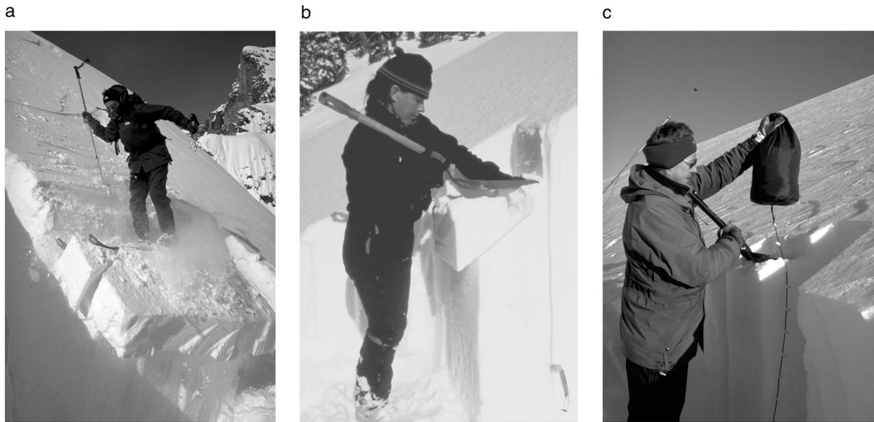
**Figure 14.** In situ snow slope stability testing usually involves isolating a snow block including a weak layer and loading the block at given steps: (a) rutschblock test, (b) compression test, and (c) stuff block test [from Schweizer and Jamieson, 2003a].
